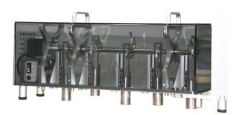
**T**M003 Tapping Machine is a rugged, self-contained sound source for making footfall noise measurements to the latest international standards (ISO140, EN 20140, ASTM E492, GB J75-84, etc.).
