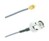
**Model CUBnnn:** 10-32 UNF (or M5) to BNC cables commonly used to connect accelerometers or other transducers to acquisition system and analyzers. Model number indicates cable length. Also available are cables suitable for high temperature environments.
